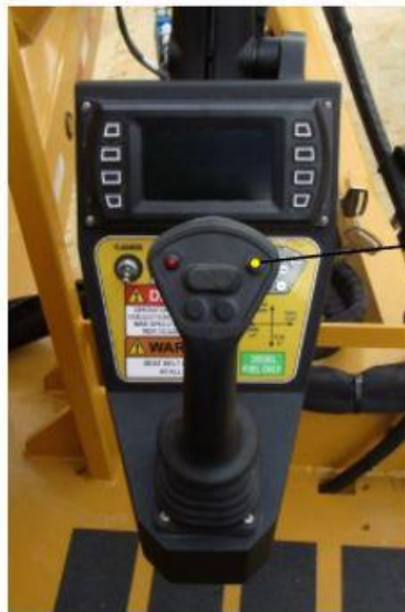
On-Off Switch - Shown On Proportional Joystick (Location On Other Models May Vary)
