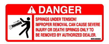
If possible, have your bonnell dealer service the canisters for you. They are under extreme pressure, and special tools may be required to remove and reassemble the spring assembly.
