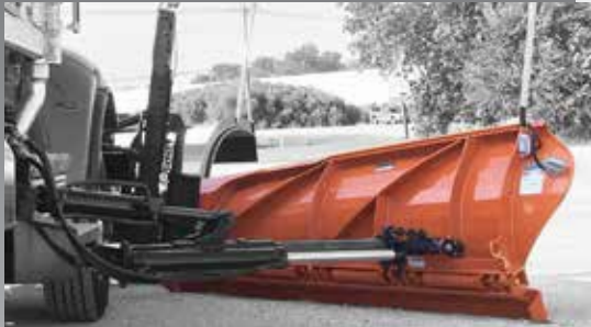
Front Mounted Patrol Wing with Trip Edge and Hydraulic Buffer Brace
