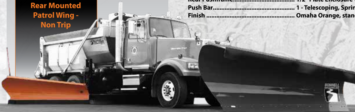
Front Mounted Patrol Wing with Trip Edge and Hydraulic Buffer Brace
